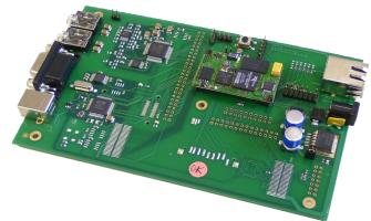
Motherboard for BFlancore, also suitable for BF561multicore
